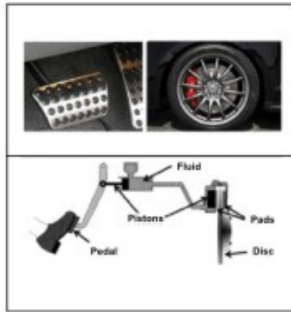
Disc Brake System
